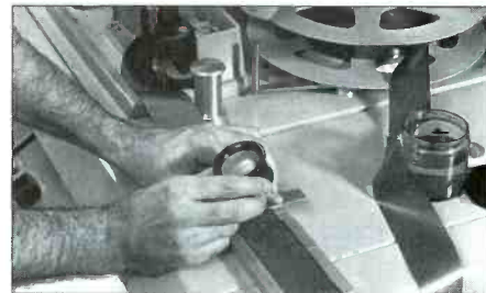
Years ago, a solution containing magnetic-sensitive particles was applied to 2-inch tape to determine where to "make the cut" with a razor blade. (Photo courtesy of Ampex.)
